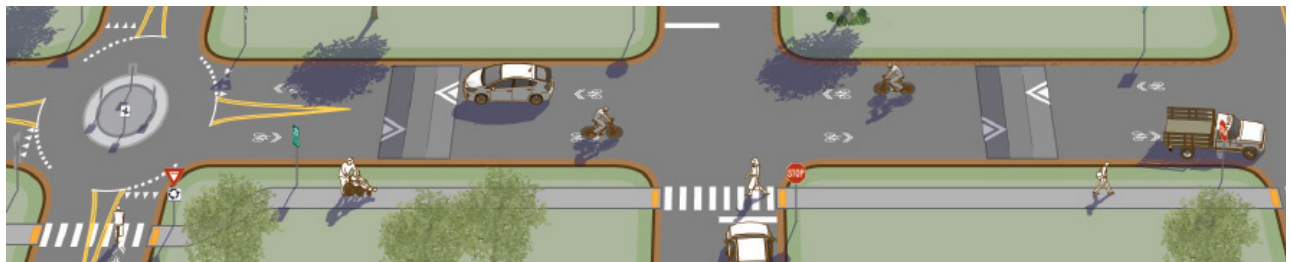
Mixed Traffic Example (Shared Lane) - Applicable to the downtown Trade St (south of Howard St) section of this project
