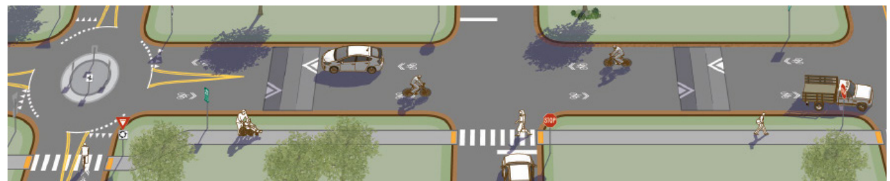
Mixed Traffic Example (Shared Lane) - Applicable to the Main St section of this project
