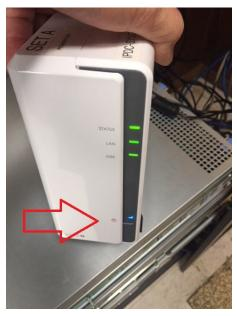
STEP 4: PUSH POWER ON SYNOLOGY UNIT STEP 5: CONFIRM LIGHTS ARE ILUMINATED ON BOTH UNITS.
